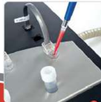
300 \mu l sample volume per analysis (mini test cell with 175 \mu l volume available for research use).
